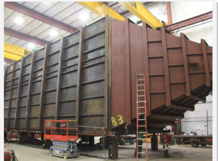
Above: Partial fabrication of the 3rd baghouse module in this 8 baghouse module project
