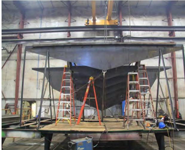
*The bow section of a marine vessel in mid-fabrication.*
